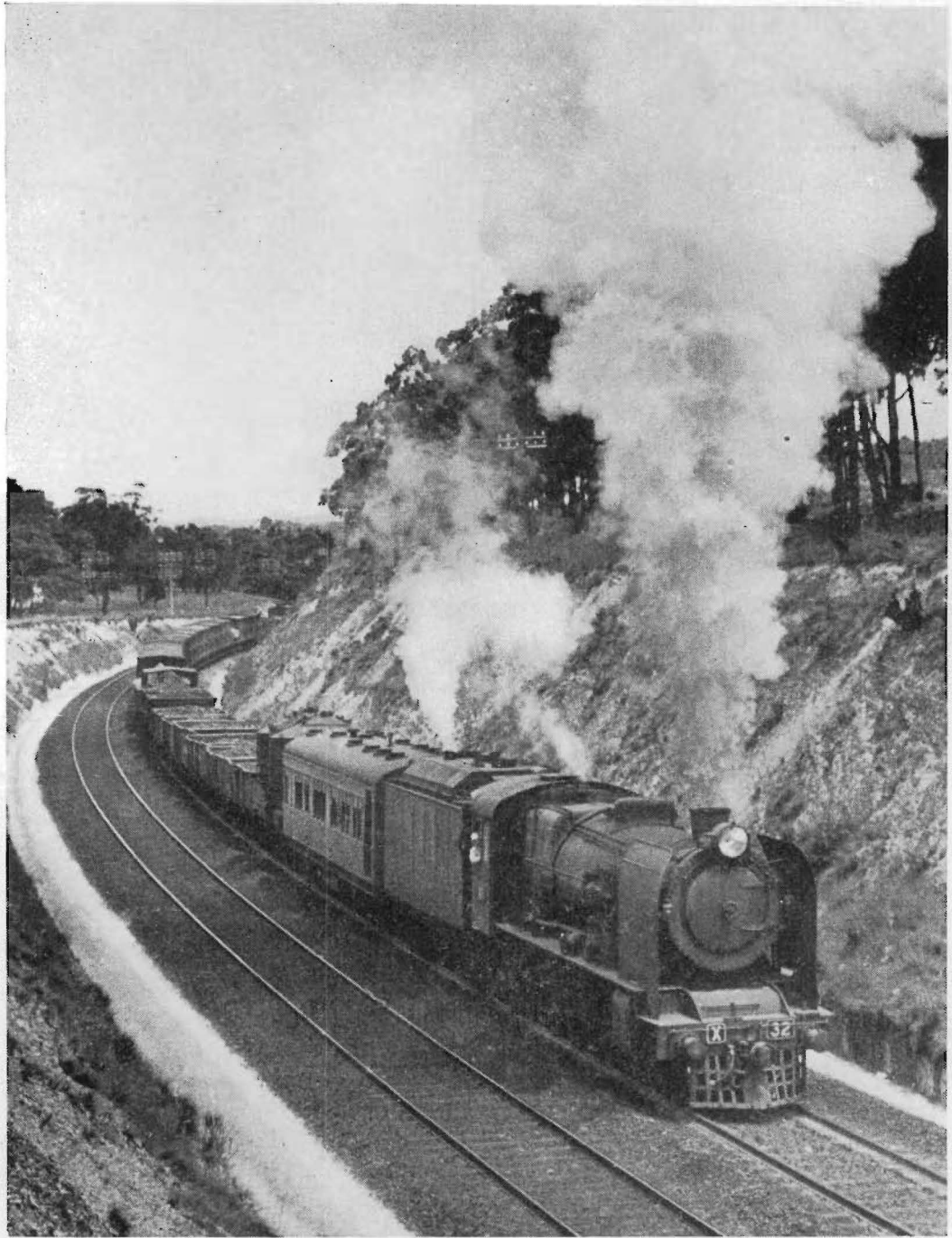
Goods train hauled by engine burning pulverised brown coal.
